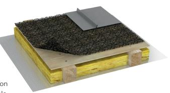
for use in ventilated and non-ventilated facades. Polypropylene multifilament acts as a separation layer and significantly improves durability of the roof by ensuring proper ventilation and condensate drainage.
