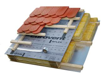
(mineral wool, fiberglass) is not required for installation – product can be installed directly on thermal insulation. The final roof covering must be assembled with batten and counter-batten. Suitable for use in nearly all types of roof coverings – recommended for cement and clay tiles as well as metal
