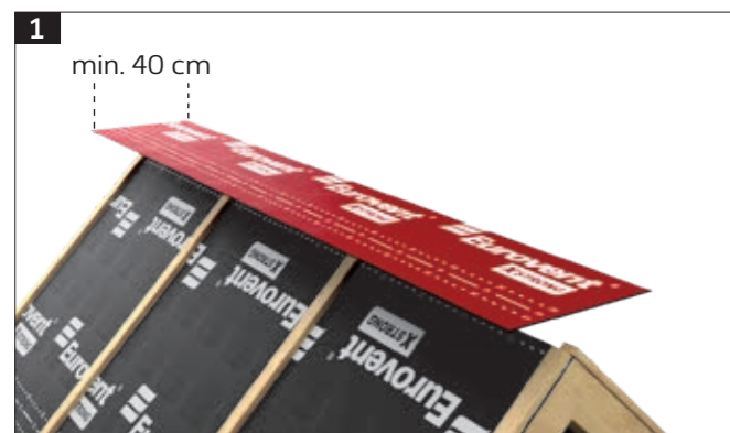
Instruction of the Eurovent® ridge tape installation
