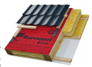
on thermal insulation. The final roof covering must be assembled with batten and counter-batten. Suitable for use in nearly all types of roof coverings – recommended for ceramic, concrete, metal roofing tiles, aluminium sheets, natural slate, etc.
