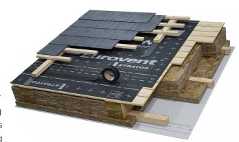
slot between the membrane and the thermal insulation (mineral wool, fiberglass) is not required for installation – the product can be installed directly on thermal insulation. The final roof covering must be assembled with batten and counter-batten. Suitable for use in nearly all types of roof coverings – recommended for ceramic, concrete, metal roofing tiles, aluminium sheets, etc.
