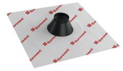
Self-adhesive sealing collar designed for sealing cables of solar installations as well as sewage, heating, and ventilation pipes in building partitions such as walls, attics, and floors. Made of highquality polyethylene laminated with acrylic adhesive and equipped with an EPDM cable grommet.
