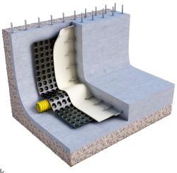
wall. Horizontal applications include protection against penetration of water in buildings where deep foundations are exposed to the risk of temporary fluctuations of subsurface water levels. It is then installed along the slope between the concrete slab and screed.
