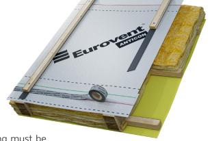
installed directly on thermal insulation. The final roof covering must be assembled with batten and counter-batten. Product is not recommended for use in fully sarked roofs.
