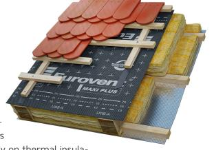
not required for installation –product can be installed directly on thermal insulation. The final roof covering must be assembled with batten and counter-batten. Suitable for use in nearly all types of roof coverings – recommended for cement and clay tiles as well as metal roofing.
